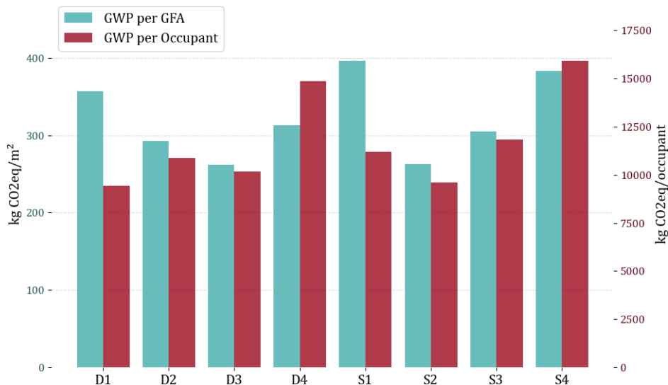
Figure 3. Global Warming Potential for the 8 buildings; results are presented for both functional units
